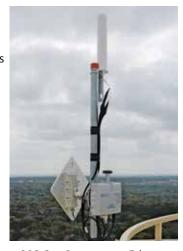
RUGGEDCOM RP100 single-port 802.3xx Power-over-Ethernet (PoE) injector, which powers the other two devices.
